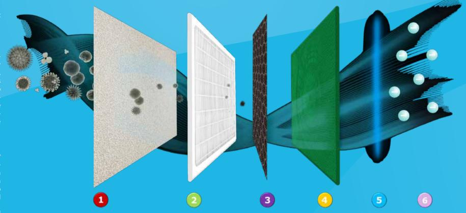
filtering gaseous impurities in the room air. The filter is capable of reducing a wide range of pollutants such as formaldehyde, benzene and various volatile organic compounds (VOC) in the air. The filter material is based on a ceramic granulate, which has been optimized by various processes.
